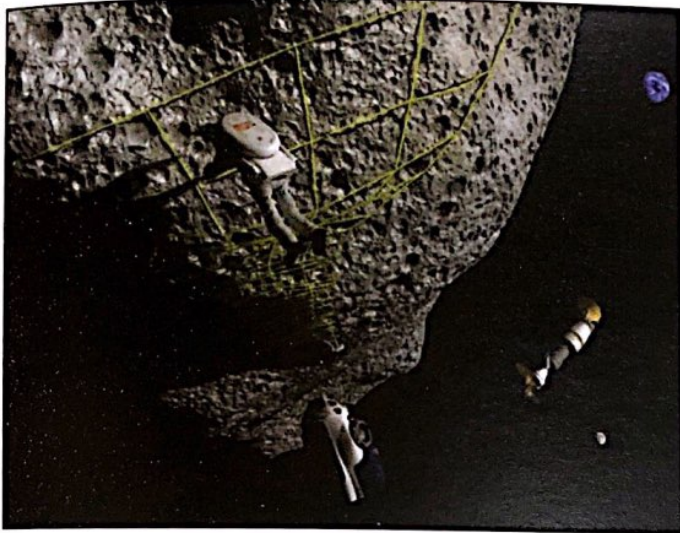
This is an illustration of a possible system for anchoring to the surface of an asteroid.
