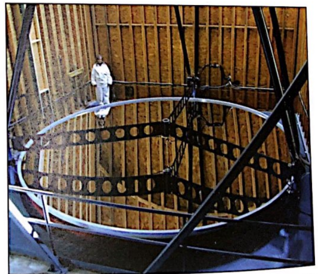
This liquid mirror telescope, the largest on Earth, is 6 meters (20 feet) across. On the Moon, undisturbed by wind or weather, the surface could be larger than a football field.
